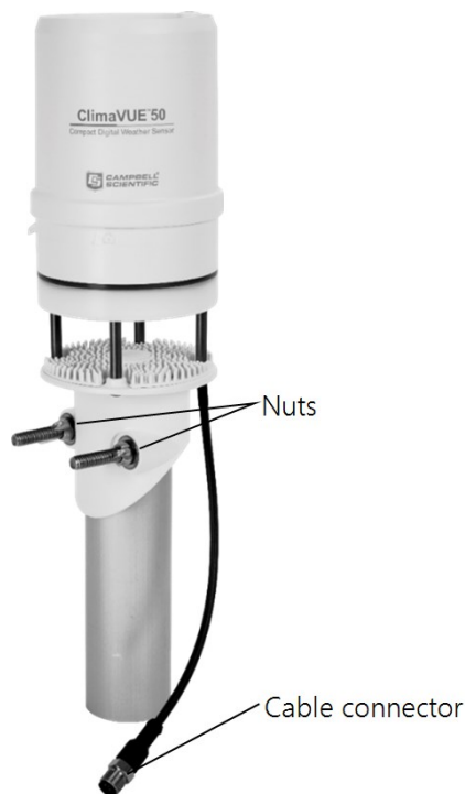
Figure 7-5. ClimavUE 50 with connector cable
